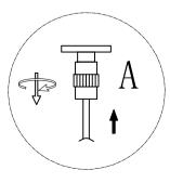
When adjusting the height of the steel wire, the telescopic metal part A toothed outer ring can only twist half a turn, and then pull it up to adjust the height!!! IMPORTANT: Test sockets with bulb before dressing the fixture.
